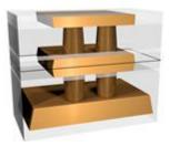
Hybrid bonding uses direct, copper-to-copper interconnects to increase the I/O density while shortening the lengths of the wiring between chiplets, thereby improving overall performance, power and cost.
