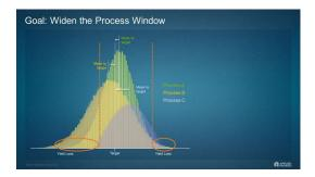
Let's look at a histogram that captures the complexity. There is a distribution for each process step. And achieving the widest process window means increasing the control of the mean and distribution of each one. As you can imagine, this requires massive amounts of data, which we call "big in-line data."
