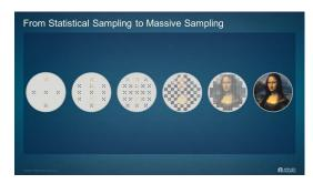
Let's illustrate how massive, across-wafer sampling can reveal patterns. Here is a small number of data points similar to the statistical die sampling used in optical overlay. You cannot notice any across-wafer variability issues. Now let's give you more samples. Thanks to the additional data, it is now clear to you that this is the Mona Lisa.
