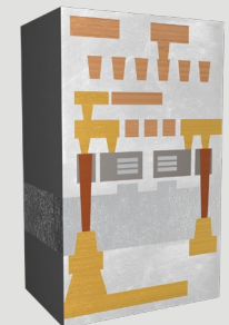
GAA with Backside Power Network
